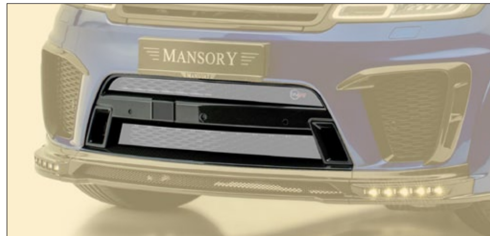
Front bumper air intake cover - With camera
