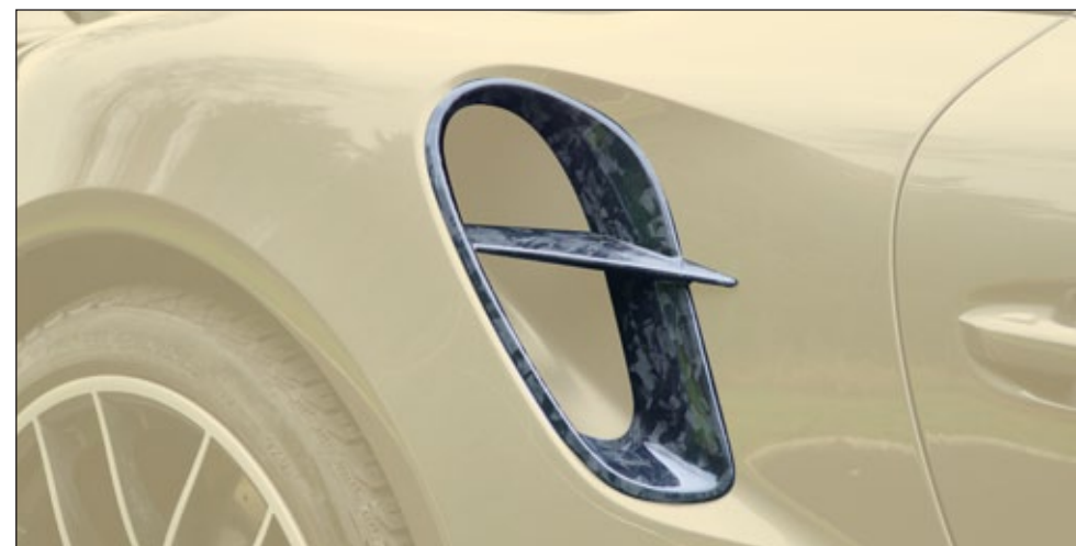
Body air intake cover for original rear bumper, 2 parts set - left & right, visible carbon fibre glossy*
