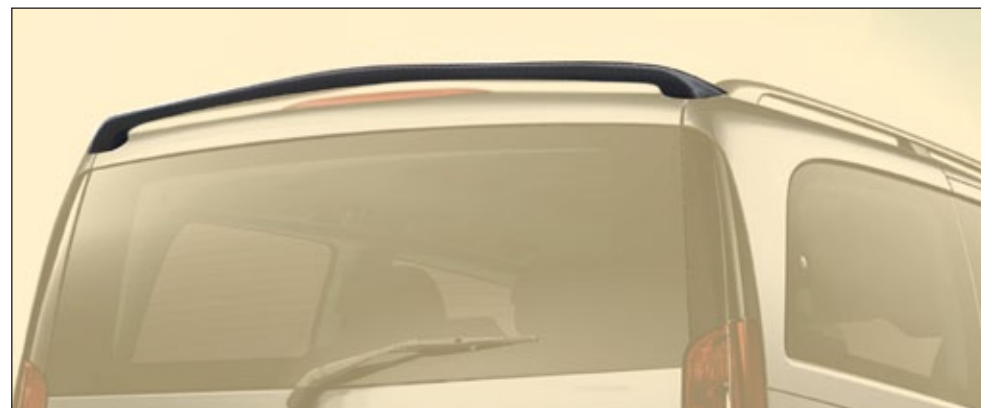
Roof spoiler exposed visible carbon fibre without clear coat
